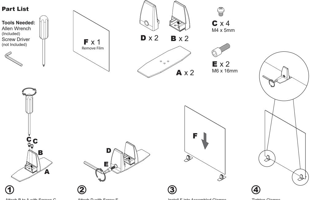
Attach B to A with Screws C
