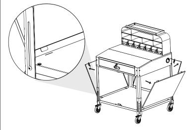
Tilt the panels to vertical and secure them in place using the locking pins.
