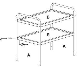
Place the cart on a level surface and tighten all of the hardware using the Allen wrench and a  $\frac{1}{2}$  or 13mm Wrench.
