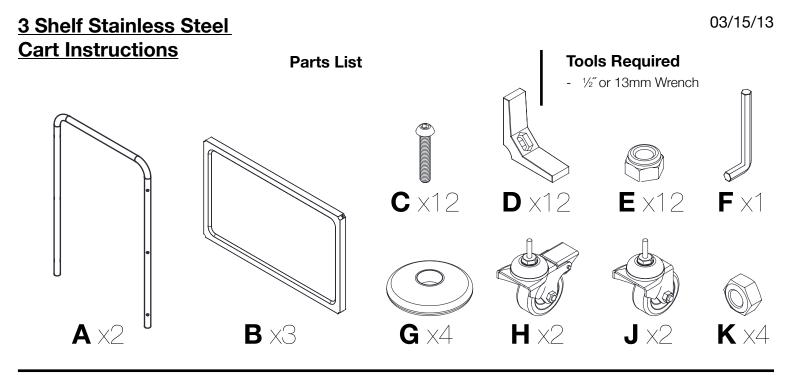
Using Allen wrench **F** and a  $\frac{1}{2}$  or 13mm Wrench, attach the top shelf to the tube frames with 4 screws **C**, 4 corner brackets **D** and 4 locking nuts **E**.
