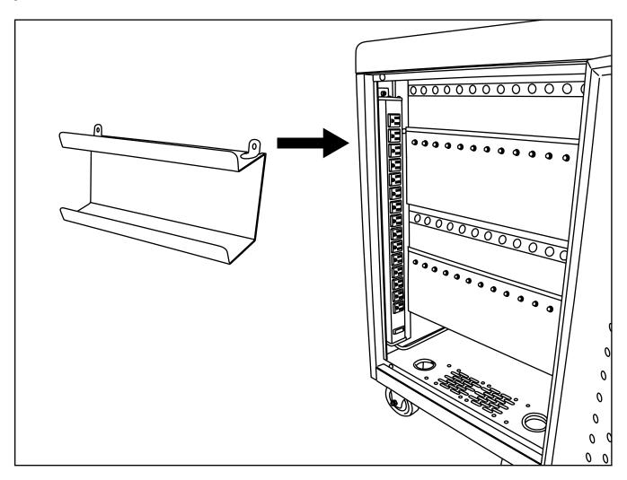
Place the nut in front of the power brick holder and tighten. Then repeat for the second Power Brick holder.
