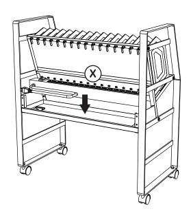
Step 8: Install the power tray back panel (H) with 4 screws (S), using a screw driver.
